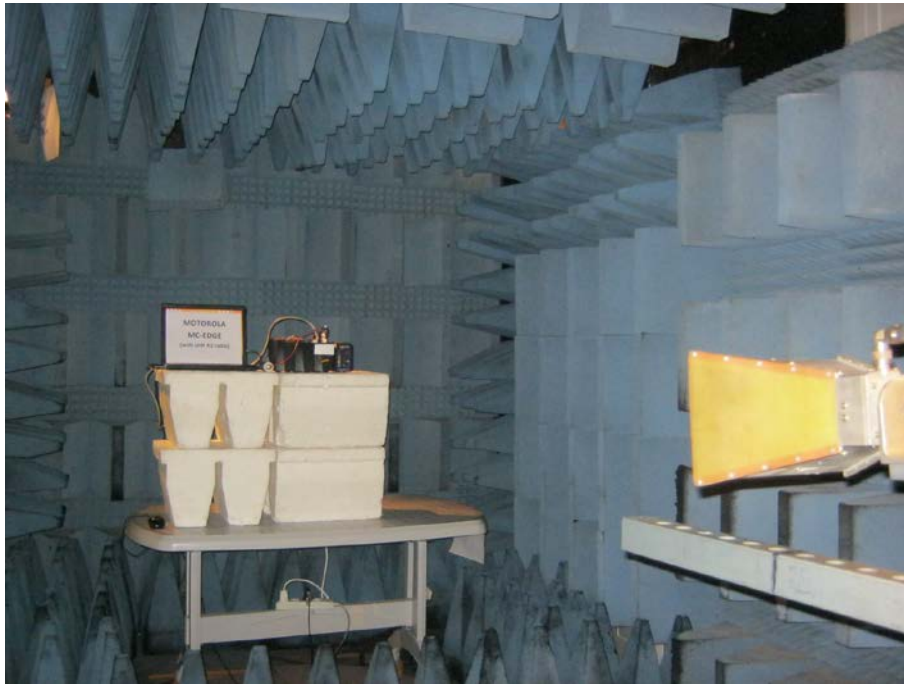
Figure 7. Radiated Emission Test, 1000-6000MHz
