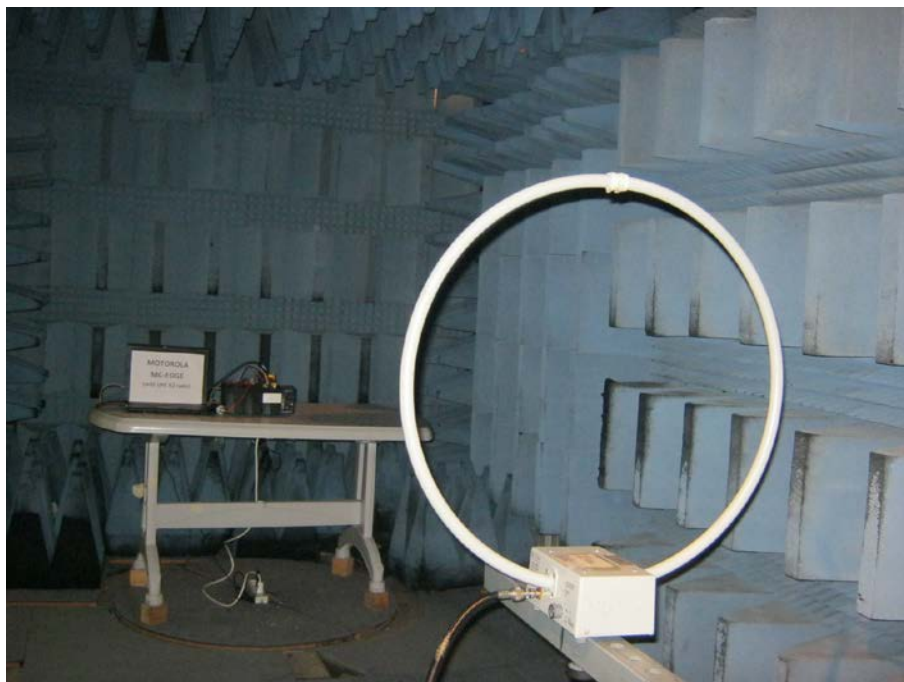
Figure 4. Radiated Emission Test, 0.009-30MHz
