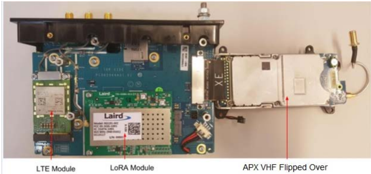
MC-EDGE Piggy Board Top View With Front Panel (APX4000 VHF Flipped over, with LORA and LTE)
