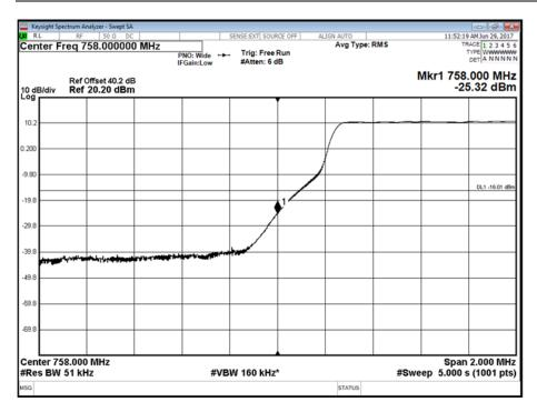
Antenna A - LTE Modulation QPSK - LTE Carrier Bandwidth 5.0 MHz - Channel Position T
