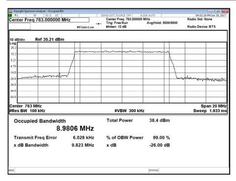
Antenna B - LTE Modulation 64QAM - LTE Carrier Bandwidth 10.0 MHz - Channel Position T
