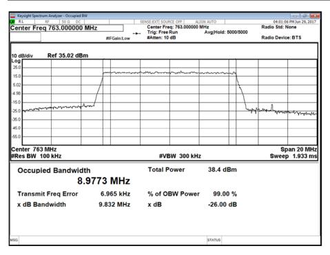
Antenna B - LTE Modulation 64QAM - LTE Carrier Bandwidth 10.0 MHz - Channel Position B
