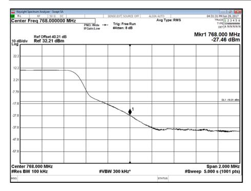
Antenna A - LTE Modulation 16QAM - LTE Carrier Bandwidth 10.0 MHz - Channel Position M
