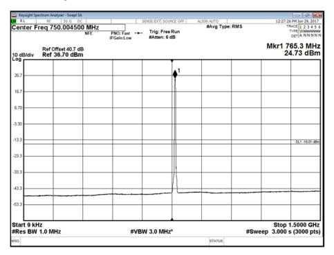
Antenna B - LTE Modulation 16QAM - LTE Carrier Bandwidth 5.0 MHz - Channel Position T - Band 2 - Range 1500 to 8000 MHz
