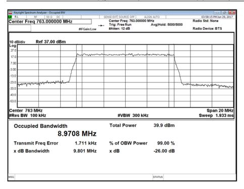
Antenna B - LTE Modulation 16QAM - LTE Carrier Bandwidth 10.0 MHz - Channel Position B
