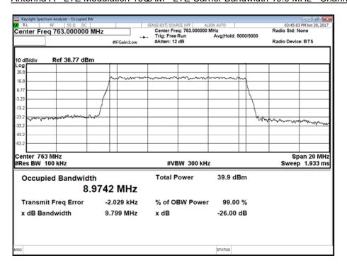
Antenna B - LTE Modulation 16QAM - LTE Carrier Bandwidth 10.0 MHz - Channel Position M
