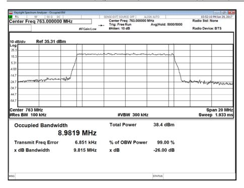
Antenna B - LTE Modulation 64QAM - LTE Carrier Bandwidth 10.0 MHz - Channel Position M
