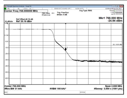
Antenna A - LTE Modulation 16QAM - LTE Carrier Bandwidth 5.0 MHz - Channel Position B
