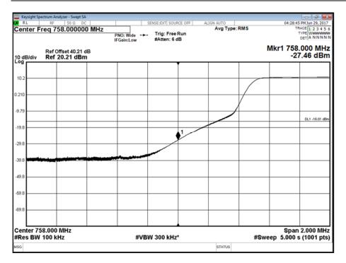
Antenna A - LTE Modulation QPSK - LTE Carrier Bandwidth 10.0 MHz - Channel Position M
