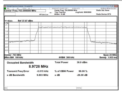
Antenna B - LTE Modulation 16QAM - LTE Carrier Bandwidth 10.0 MHz - Channel Position T
