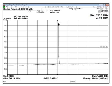
Antenna A - LTE Modulation QPSK - LTE Carrier Bandwidth 5.0 MHz - Channel Position T - Band 2 - Range 1500 to 8000 MHz
