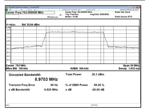
Antenna B - LTE Modulation QPSK - LTE Carrier Bandwidth 10.0 MHz - Channel Position T
