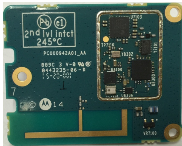
GPS/BT/Wifi board without shield (Bottom)
