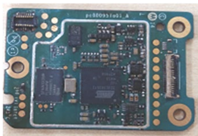
GOB board without shield (Bottom)
