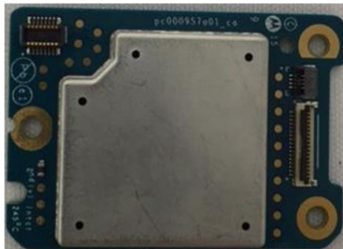
GOB board with shield (Bottom)
