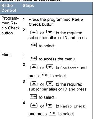
The display shows the Target Alias, indicating the request is in progress. The LED lights up solid green.
