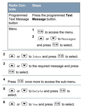
The display shows Message Deleted, and the screen returns to the Inbox.
