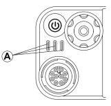
Blinking red Radio is transmitting at low battery condition, receiving or sending an emergency transmission, has failed the self-test upon powering up, or has moved out of range if radio is configured with Auto-Range Transponder System.
