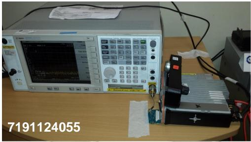
Spectrum Bandwidth (6dB Bandwidth Measurement) Test Setup
