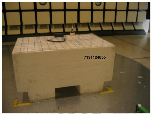
Radiated Emissions Test Setup (Front View)
