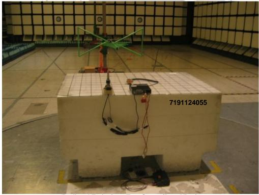
Radiated Emissions Test Setup (Rear View)
