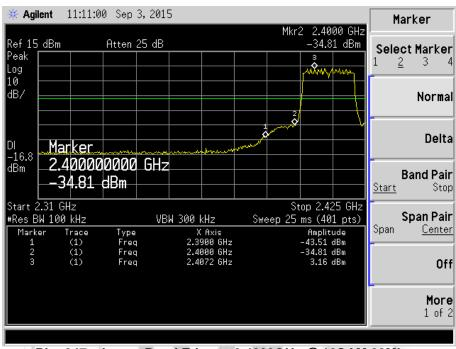
Plot 347 - Lower Band Edge at 2.4000GHz @ 16QAM 39Mbps
