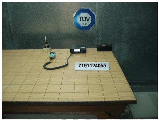
Conducted Emissions Test Setup (Front View)
