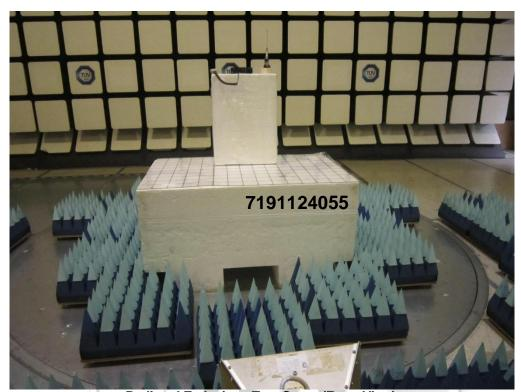
Radiated Emissions Test Setup (Front View)
