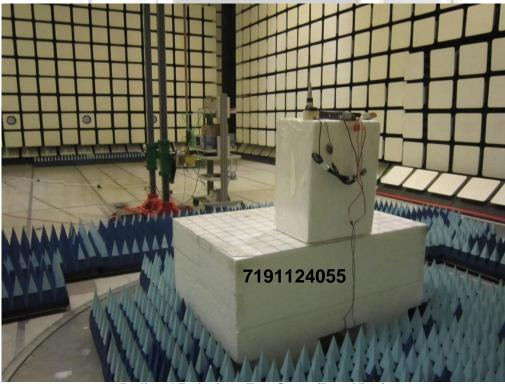
Radiated Emissions Test Setup (Rear View)
