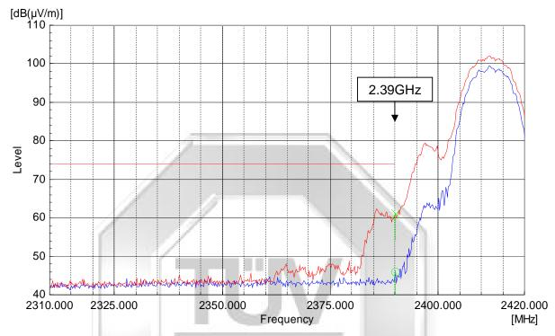
Plot 355 - Peak Plot at Lower Band Edge at 2.4000GHz @ CCK 11Mbps
