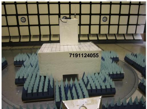
Band Edge Compliance (Radiated) Test Setup
