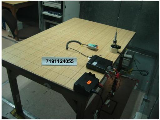
**Conducted Emissions Test Setup (Rear View)**
