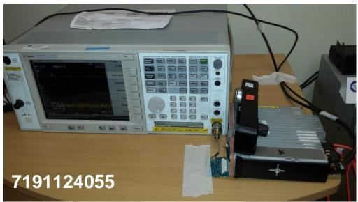
**Peak Power Spectral Density Test Setup**
