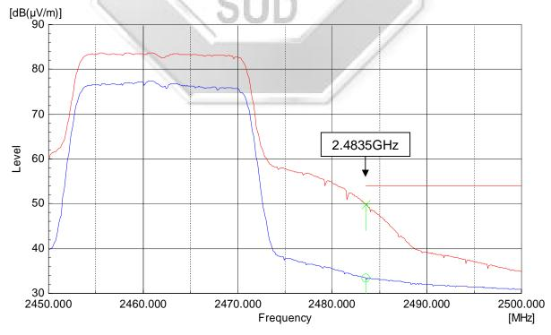
Plot 370 - Average Plot at Upper Band Edge at 2.4835GHz @ 64QAM 65Mbps
