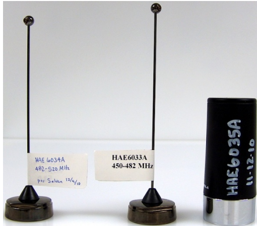
UHF Antenna kit numbers, from left to right: HAE6034A, HAE6033A & HAE6035A
