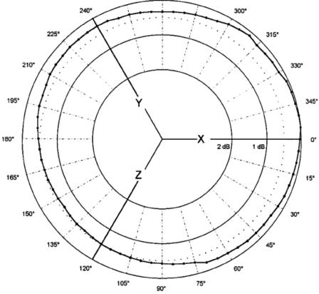
Isotropic response measured in a 20 V/m field at 400 MHz
