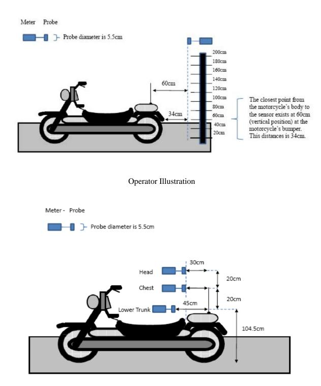
Note that the Lower Trunk distance measurement distance from the antenna (45cm) allows achieving 20cm distance from reradiating objects.
