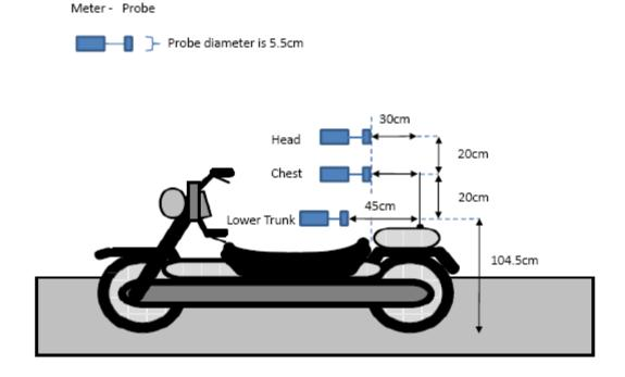
Note that the Lower Trunk distance measurement distance from the antenna (45cm) allows achieving 20cm distance from reradiating objects.
