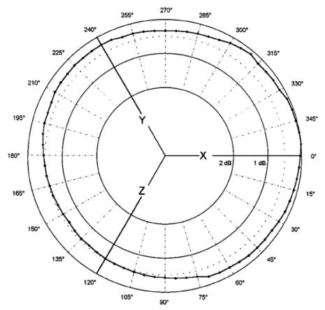
· Isotropic response measured in a 20 V/m field at 400 MHz
