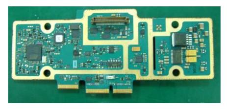
Controller board with Shields (Top)
