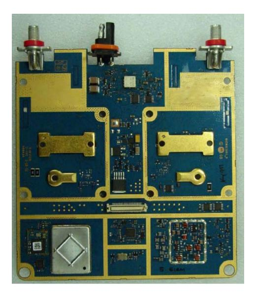
RF board without Shields (Bottom)
