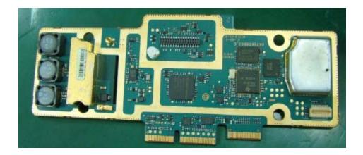
Controller board with Shields (Bottom)
