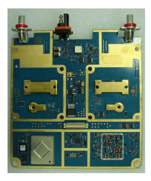
RF board with Shields (Bottom)
