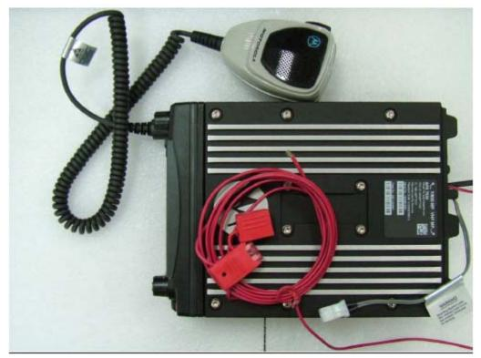
TOP VIEW WITH MICROPHONE AND REAR ACCESSORY CABLE
