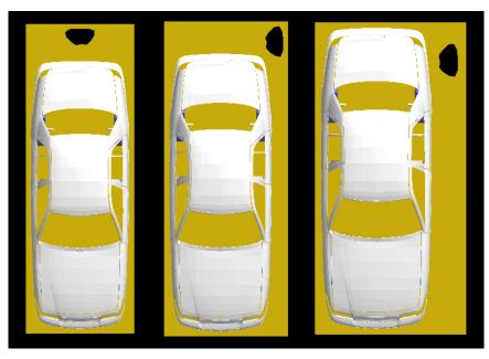
Figure 2: Top view of bystander exposure model four different locations relative to the vehicle model that replicate the measurement conditions.
