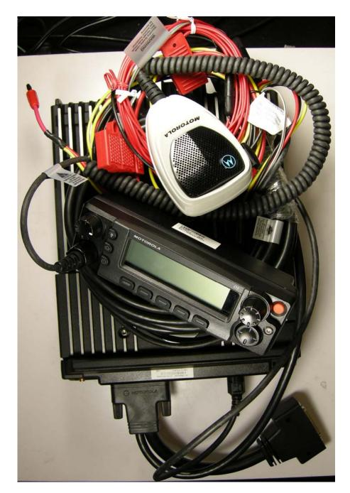
TOP VIEW WITH MICROPHONE, CONTROL HEAD AND CABLES
