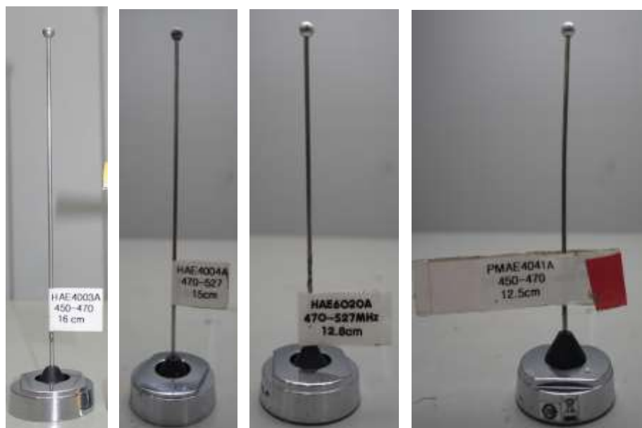
UHF2 Antenna kit numbers, from left to right HAE4003A, HAE4004A, HAE6020A, PMAE4041A
