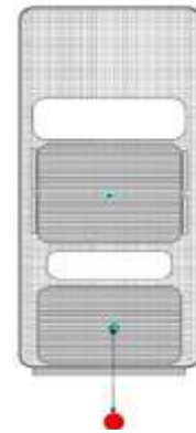
Test measurement setup for Bystander, trunk mount antenna behind vehicle
