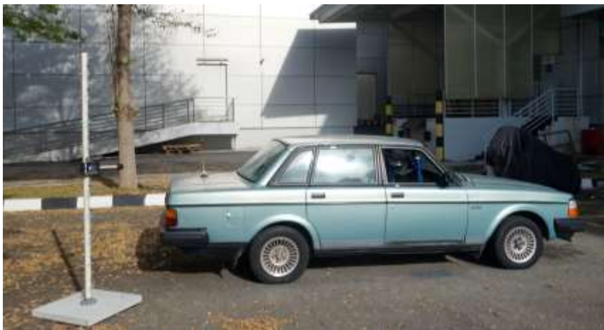
Test measurement setup for Bystander 45 degree (diagonal) trunk mount antenna
