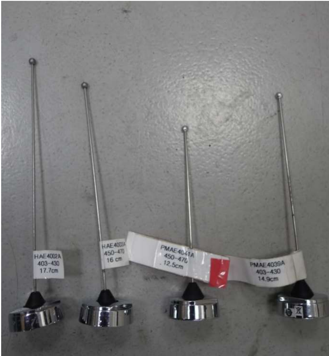
UHF Antenna kit numbers, from left to right HAE4002A, HAE4003, PMAE4039A, PMAE4041A
