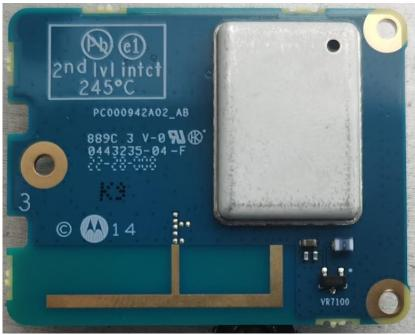
**Expansion board with shield (Bottom)**
