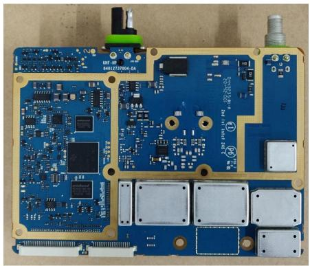
RF board with Shields (Bottom)
