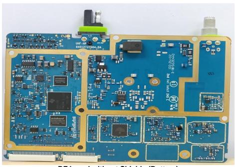
RF board without Shields (Bottom)
