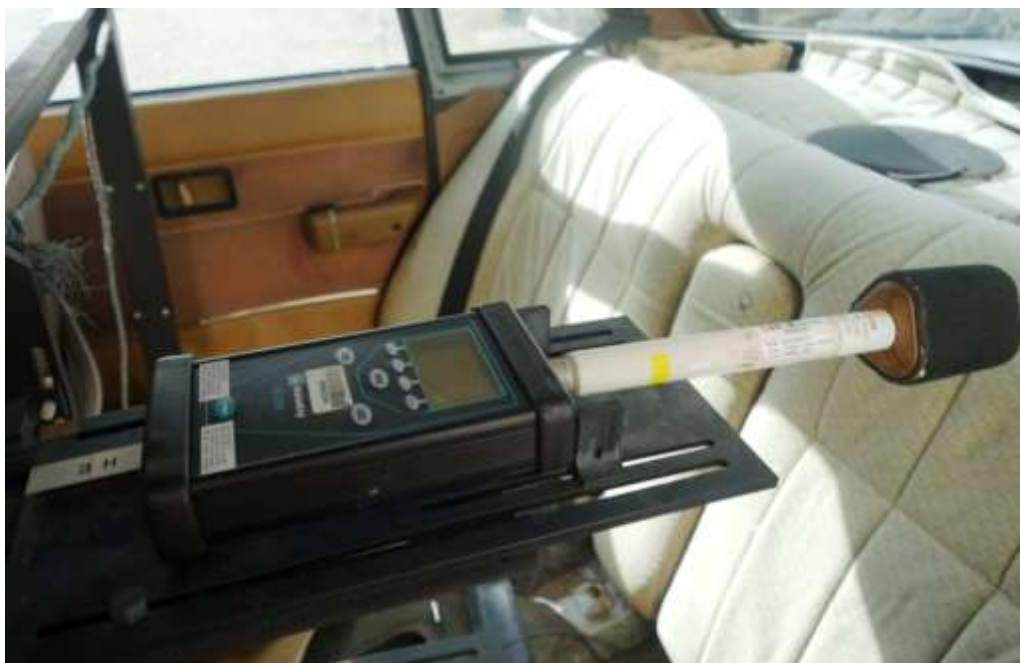
Test measurement setup for Passenger Back
