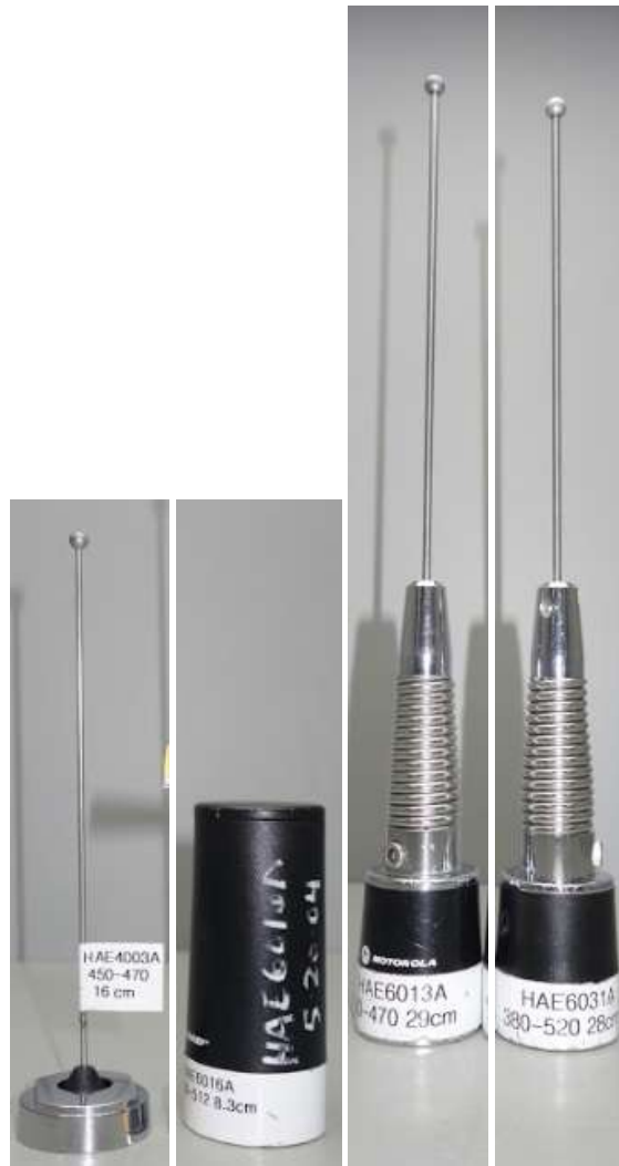
UHF R2 Antenna kit numbers: (From Left to Right) HAE4003A, HAE6016A, HAE6013A, HAE6031A
