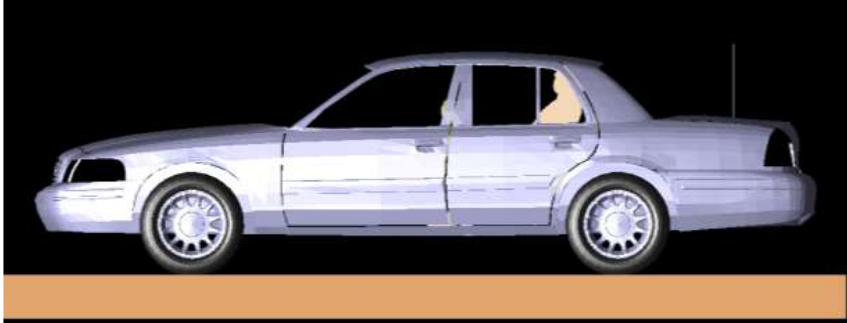
Passenger model in the center back-seat of vehicle equipped with a trunk-mount quarter-wave monopole antenna operating at VHF (150 MHz).
