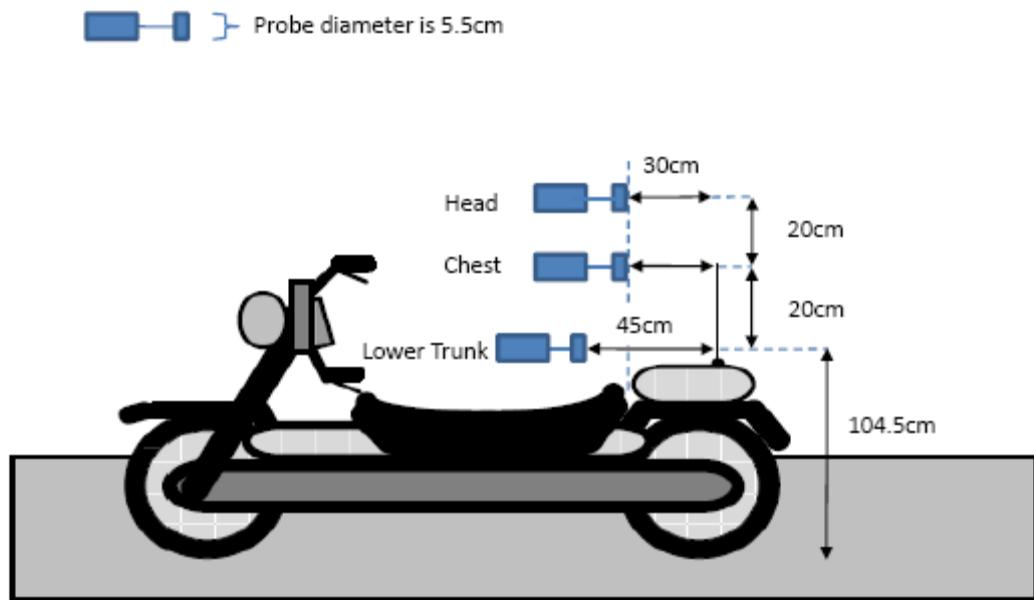
Note that the Lower Trunk measurement distance (45cm) from the antenna is to achieve 20cm distance from reradiating objects.
