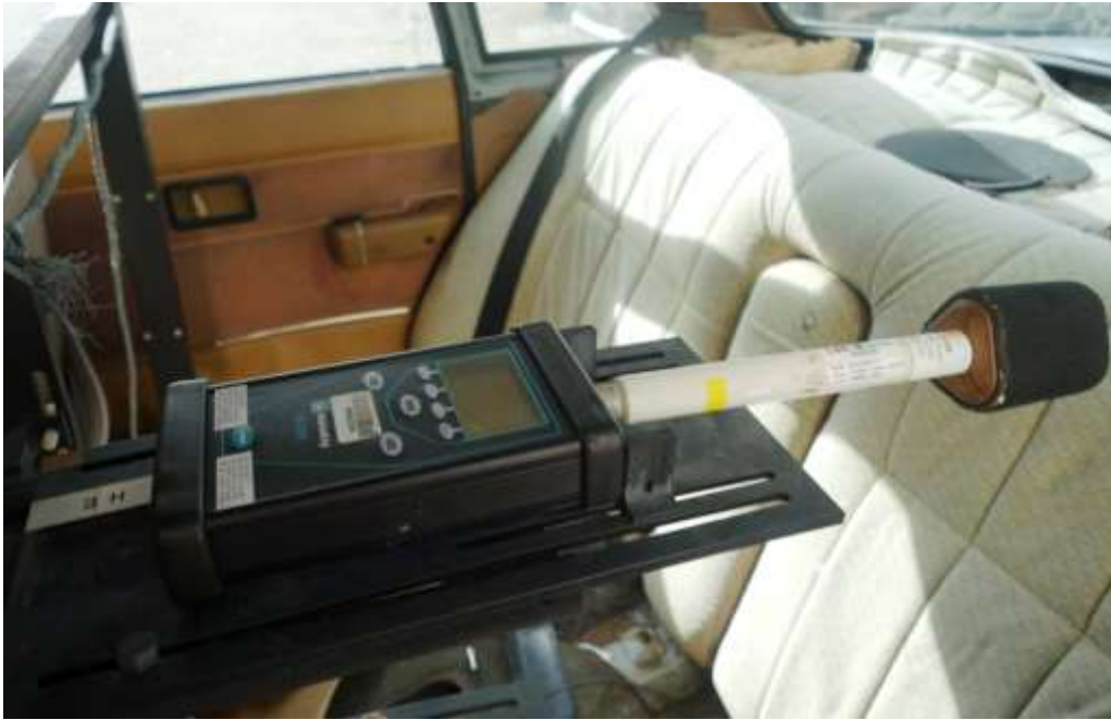
Test measurement setup for Passenger Back
