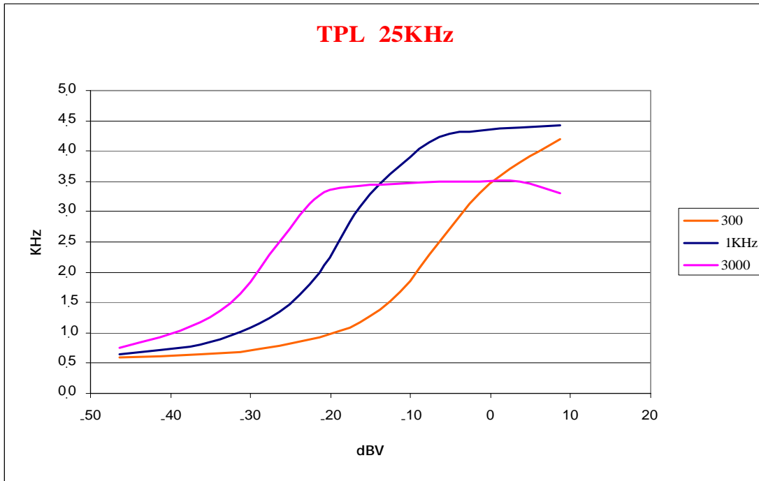
Figure 6D-5: 25 KHz Channel Spacing, Tone Private Line (TPL) Mode
