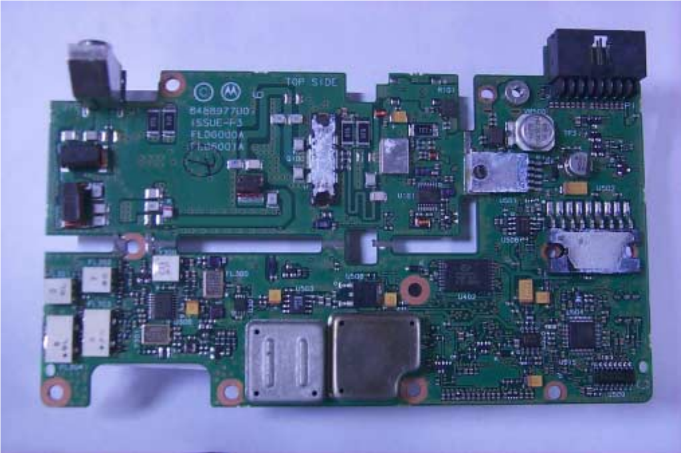
Figure 9-3: Top Side of PCB with shields.
