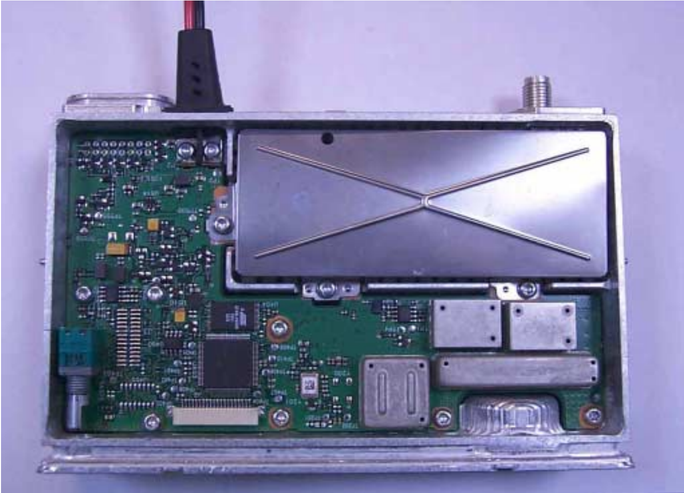
Figure 9-6: Top View of PCB placed in chassis with shield covering transmitter section.
