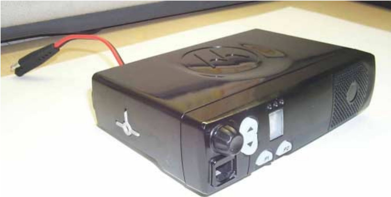
Figure 3-1: Front and side views of complete radio.
