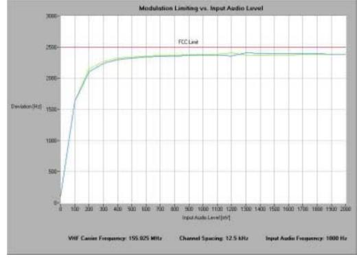
1 kHz test tone. 12.5 kHz channel spacing. Measured at 155.025 MHz.
