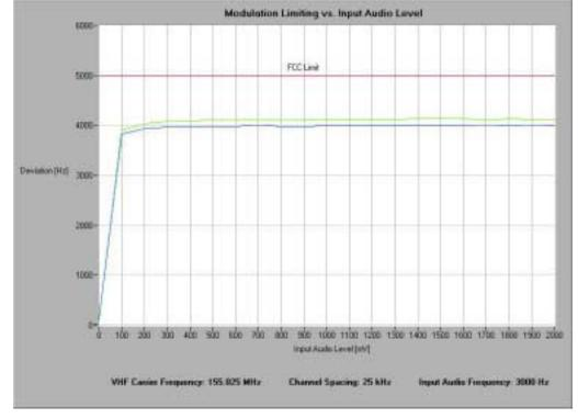
3 kHz test tone. 25 kHz channel spacing. Measured at 155.025 MHz.
