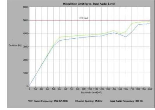
300 Hz test tone. 25 kHz channel spacing. Measured at 155.025 MHz.
