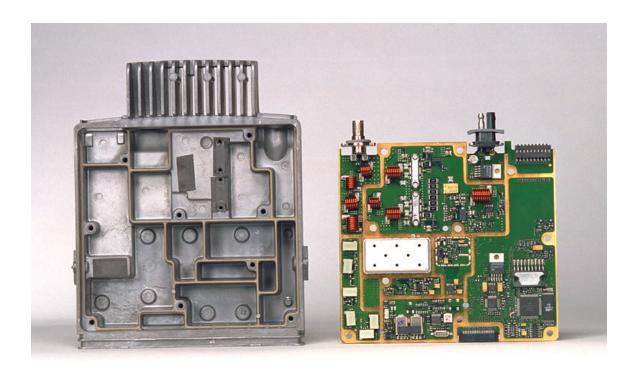
TOP VIEW OF CHASSIS, WITH CIRCUIT BOARD REMOVED (BOTTOM SIDE OF CIRCUIT BOARD VISIBLE)
