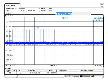
Peak of -46.50dBm, with losses at combiners factoring antenna gain to be 15.81dB, therefore level going into antenna port is -62.31dBm which exceeds threshold level of -64dBm for successful detection.
