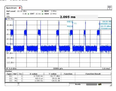
The resulting plot data was extracted and post processed, giving a duty cycle of 20.14%.
