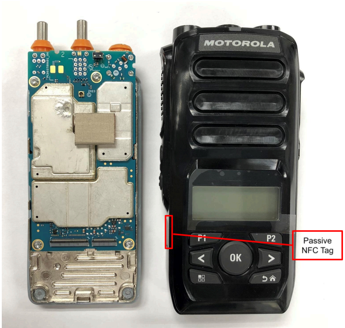
RF boards with chassis and housing for (Front Side) of LKP Model
