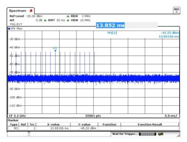
Peak of -45.22dBm, with losses at combiners factoring antenna gain to be 15.81dB, therefore level going into antenna port is -61.03dBm which exceeds threshold level of -64dBm for successful detection.
