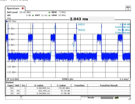
The resulting plot data was extracted and post processed, giving a duty cycle of 20.68%.
