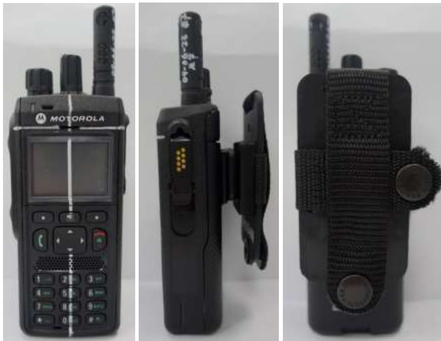
PMLN5004B w/ GMLN5401A with DUT: Front, side and back views (left to right)
