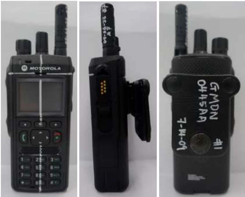
PMLN8025A w/ GMDN0445AA with DUT: Front, side and back views (left to right)
