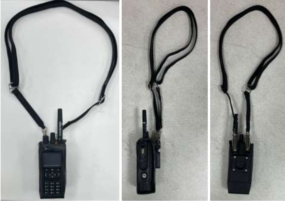
PMLN5885B w/ NTN5243A with DUT: Front, side and back views (left to right)
