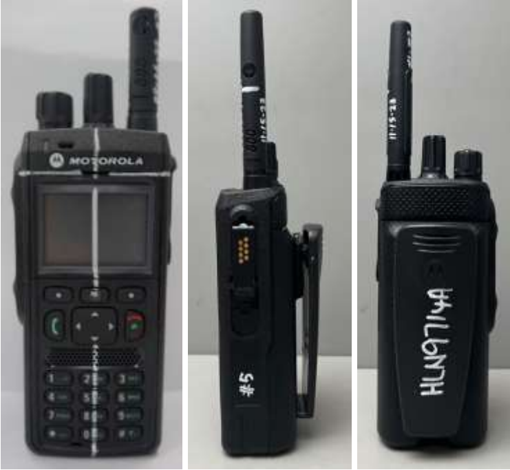
HLN9714A with DUT: Front, side and back views (left to right)
