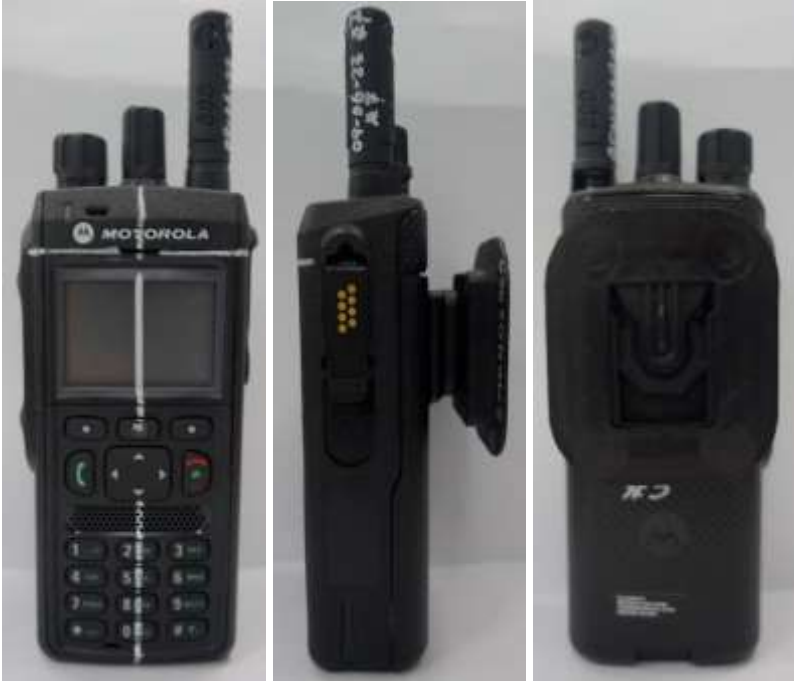
PMLN5004B w/ GMDN0386A with DUT: Front, side and back views (left to right)
