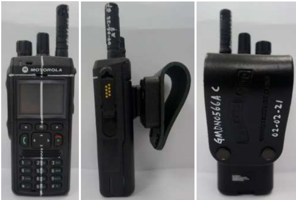
PMLN5004B w/ GMDN0566AC with DUT: Front, side and back views (left to right)
