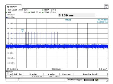
Peak of -46.77dBm, with losses at combiners factoring antenna gain to be 15.81dB, therefore level going into antenna port is -62.58dBm which exceeds threshold level of -64dBm for successful detection.
