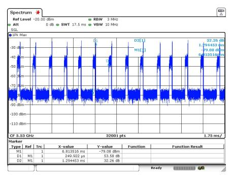
The resulting plot data was extracted and post processed, giving a duty cycle of 19.31%.
