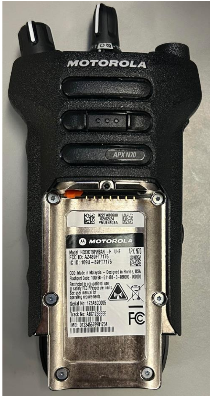
Back View (FCC/IC label) location (Model : H35XDT9PW8AN-H )
