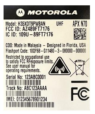
Figure 1: FCC/IC Label for APX N70
