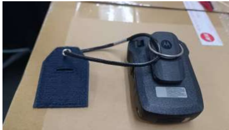
*Tethering accessory (left) hooked to the swivel clip (right)
