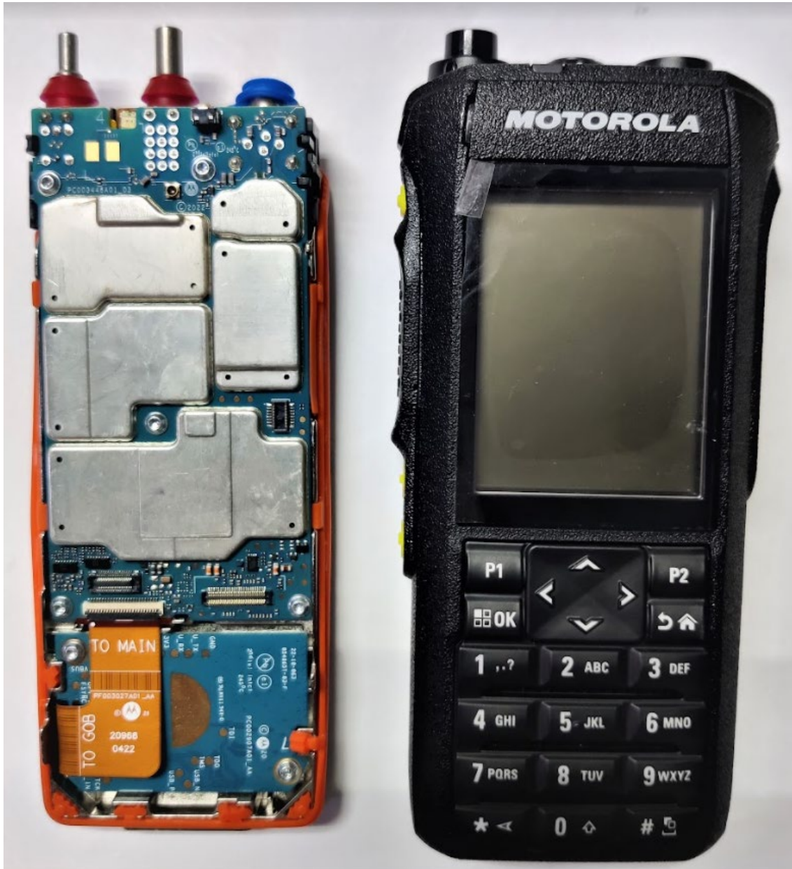
RF board with chassis and housing (front side) of TIA FKP Model
