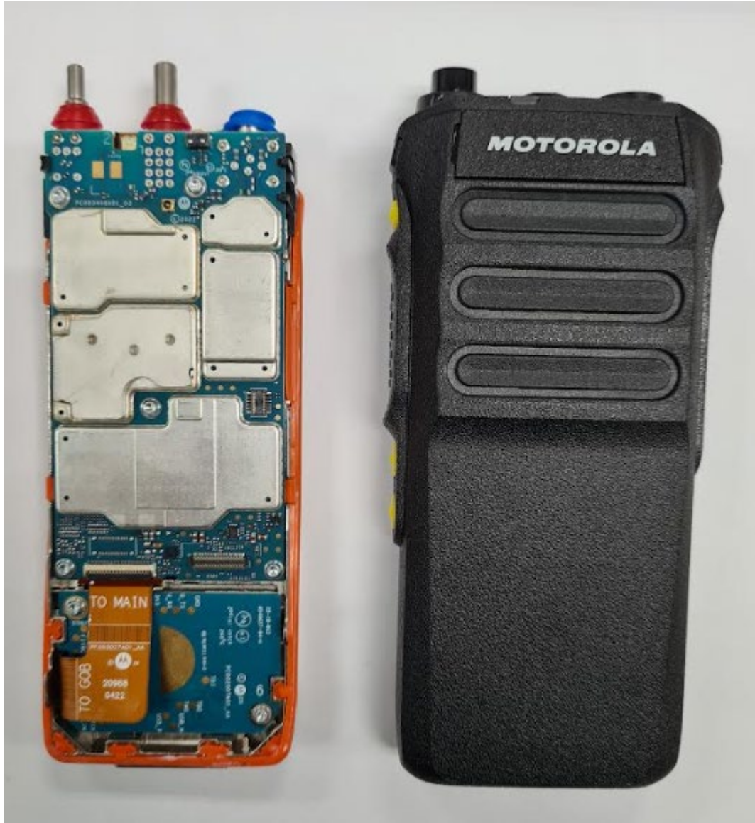
RF board with chassis and housing (front side) of TIA NKP Model
