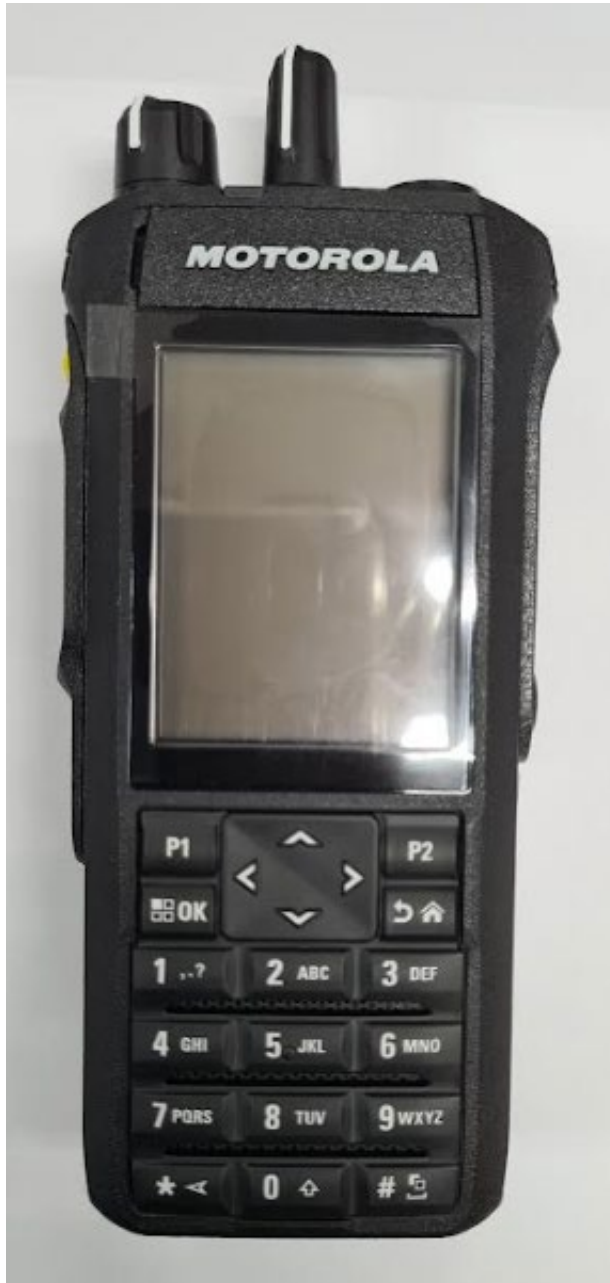
Front View of TIA Full Keypad with Display Model (R7)
