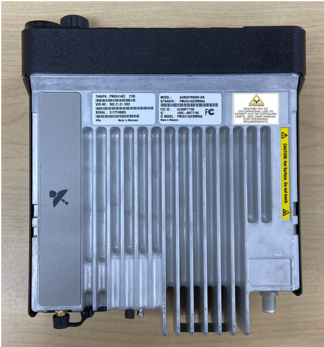
Bottom view (FCC/IC Label Location) - same for XPR 5550e Color Display and XPR 5350e Numeric Display
