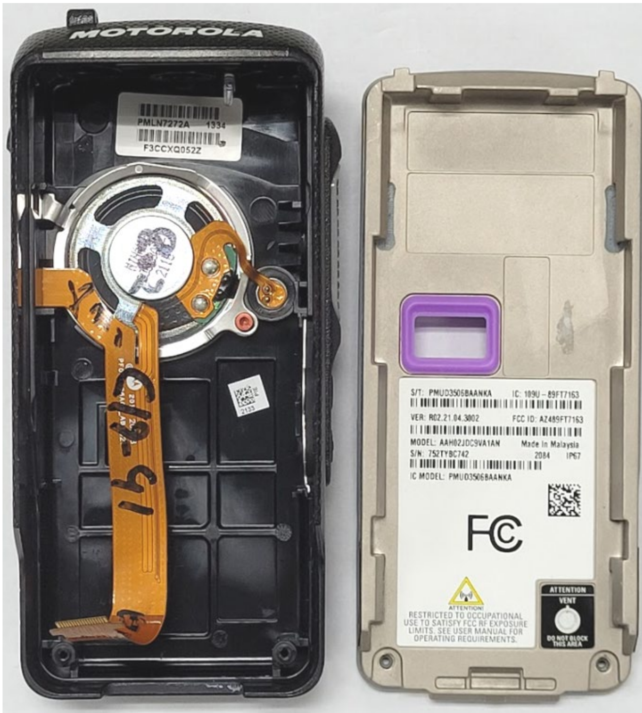
Chassis and housing (Back Side) NKP TIA4950
