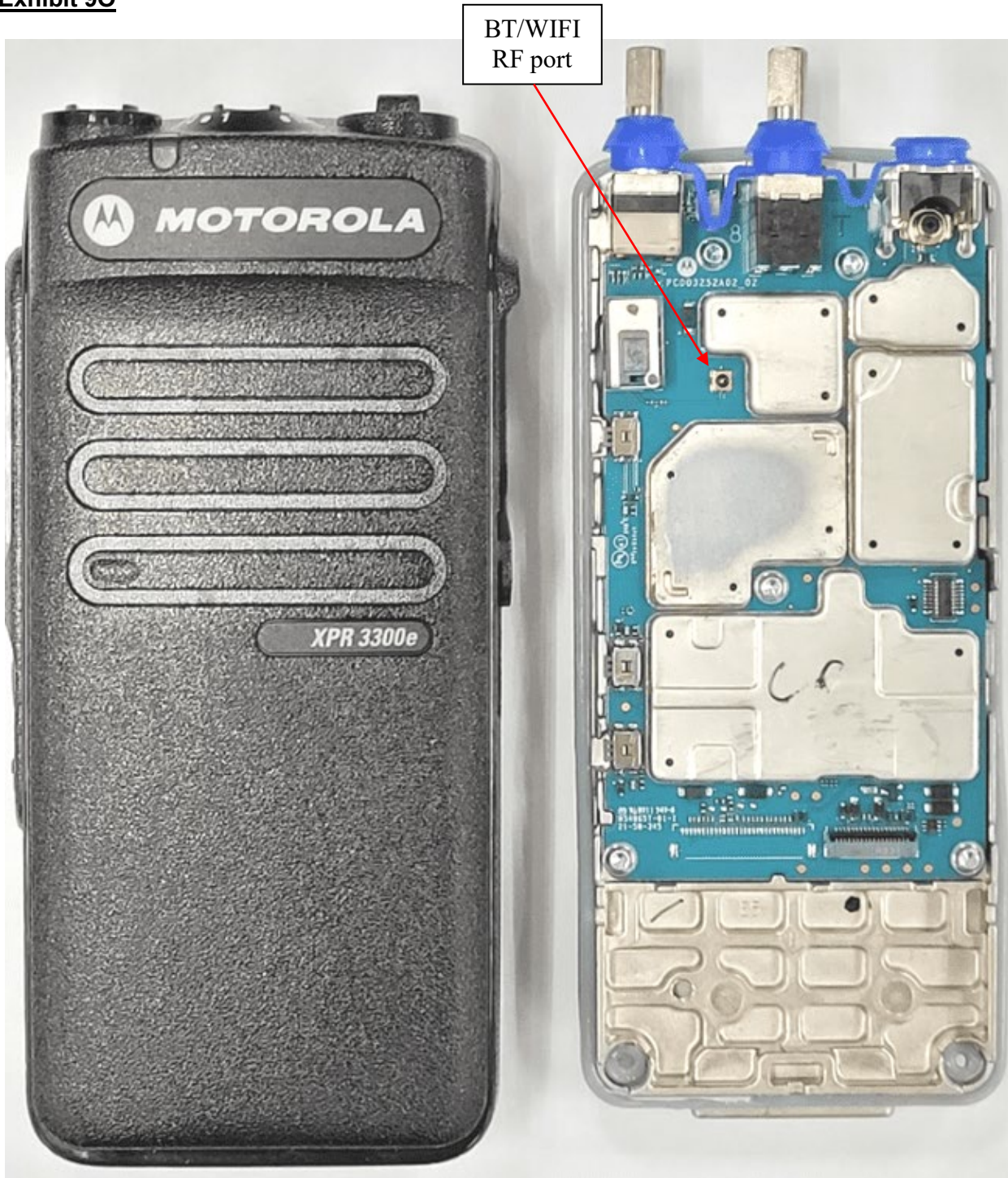
RF boards with chassis and housing (Front Side) NKP TIA4950
