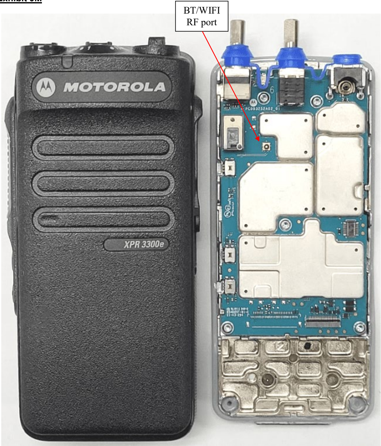
RF boards with chassis and housing (Front Side) NKP Non-TIA4950
