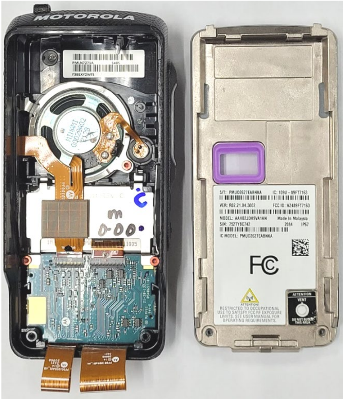
Chassis and housing (Back Side) LKP Non-TIA4950
