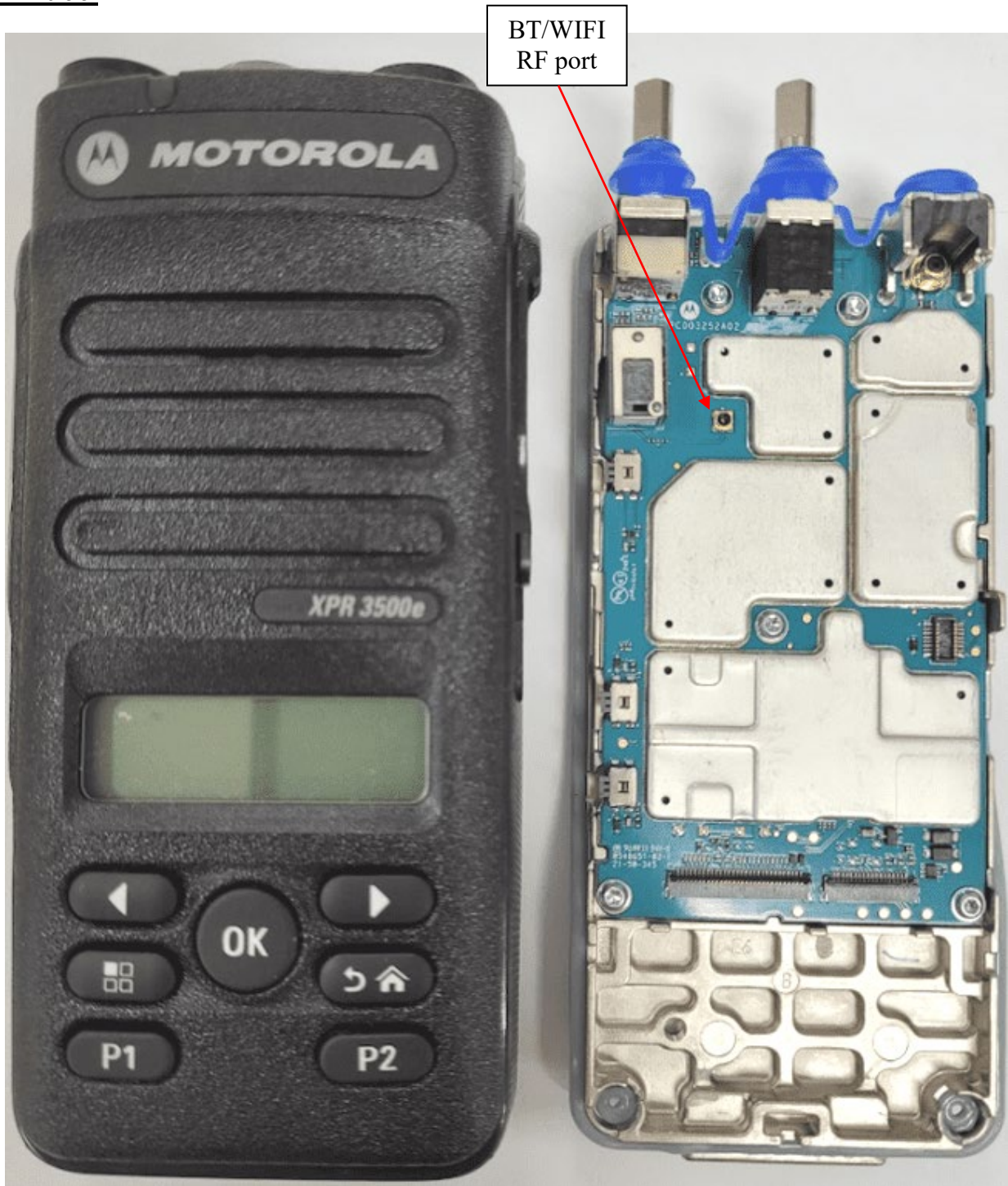
RF boards with chassis and housing (Front Side) LKP Non-TIA4950
