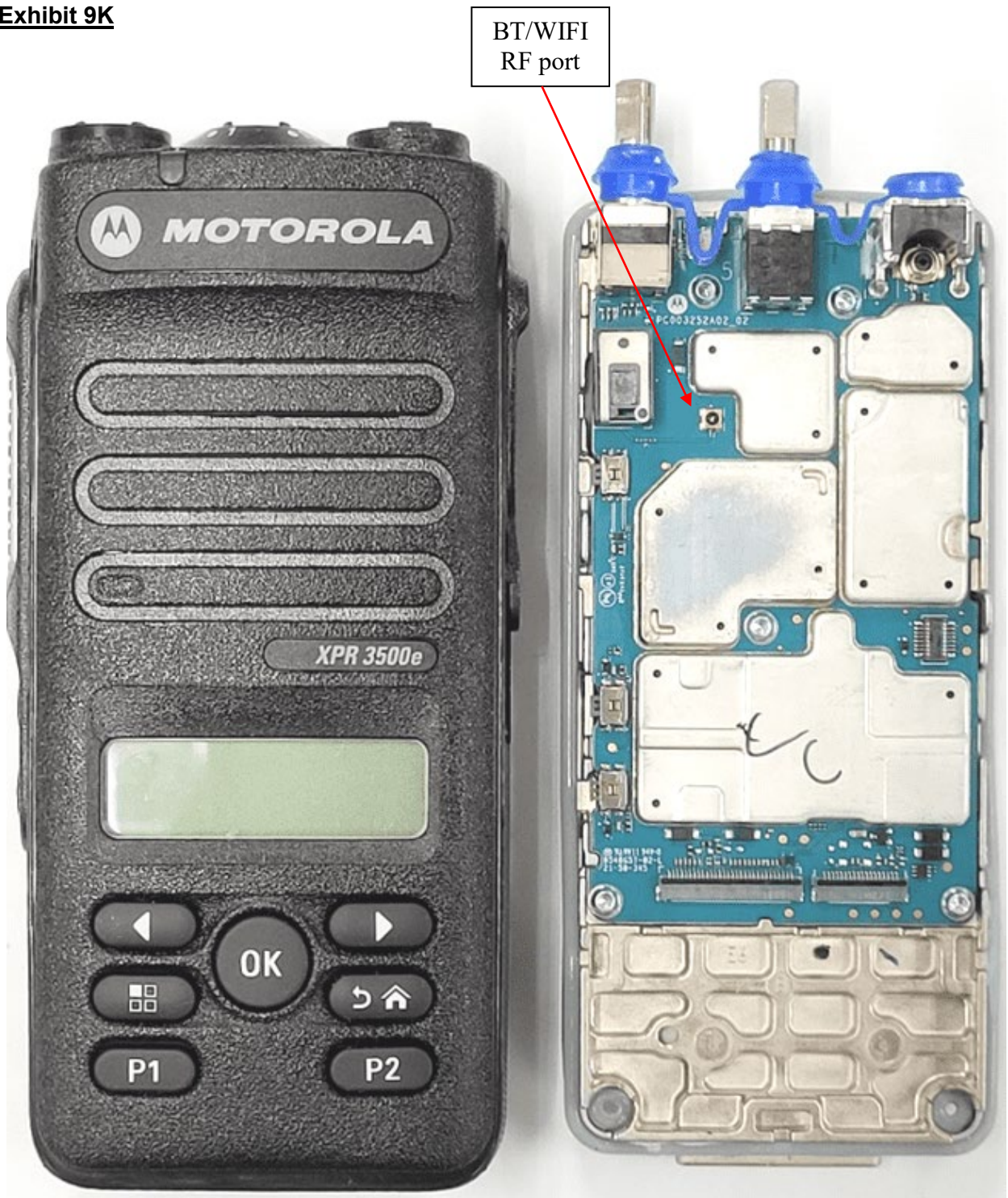
RF boards with chassis and housing (Front Side) LKP TIA4950
