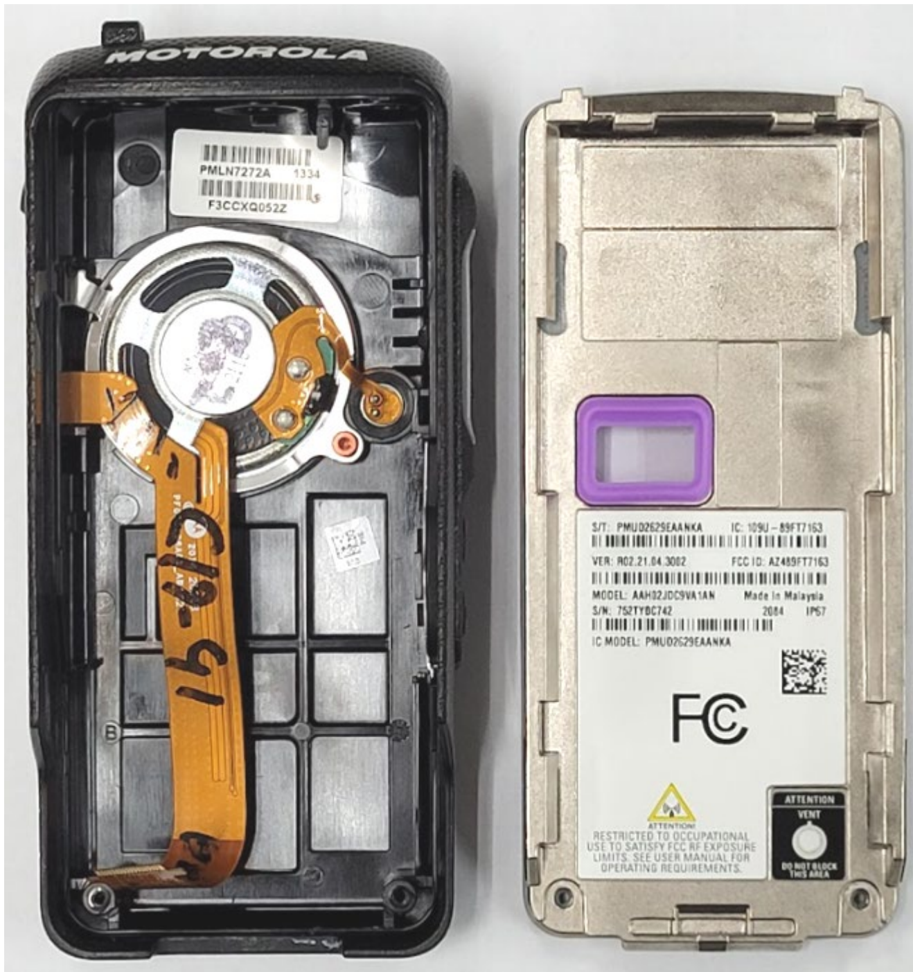
Chassis and housing (Back Side) NKP Non-TIA4950
