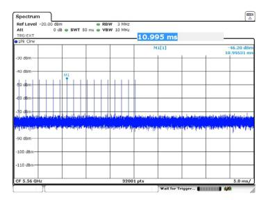
Peak of -46.20dBm, with losses at combiners factoring antenna gain to be 15.81dB, therefore level going into antenna port is -62.01dBm which exceeds threshold level of -64dBm for successful detection.
