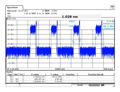
The resulting plot data was extracted and post processed, giving a duty cycle of 28.8%.
