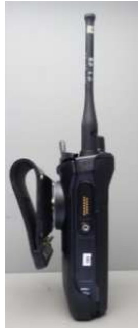
DUT Side View Body Worn PMLN8127A with Belt Loop PMLN5409A
