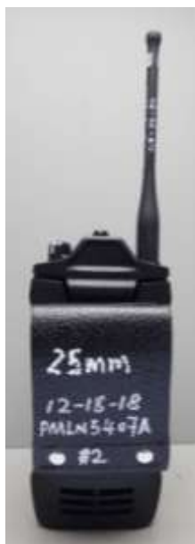
DUT Front View Body Worn PMLN8127A with Belt Loop PMLN5407A
