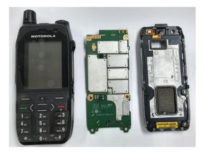
RF Board with Chassis and Housing (Front Side), Model MXP600
