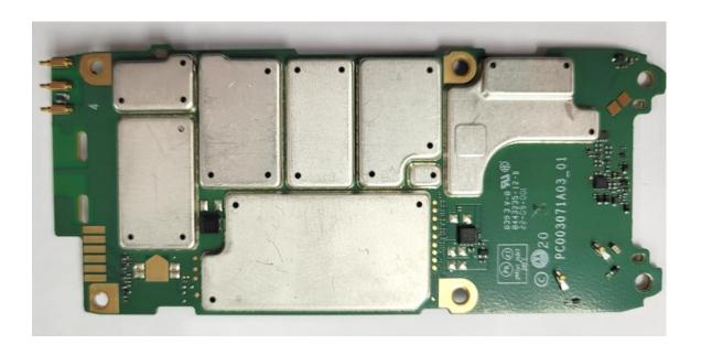
RF Board with Shields (Top), Model MXP600
