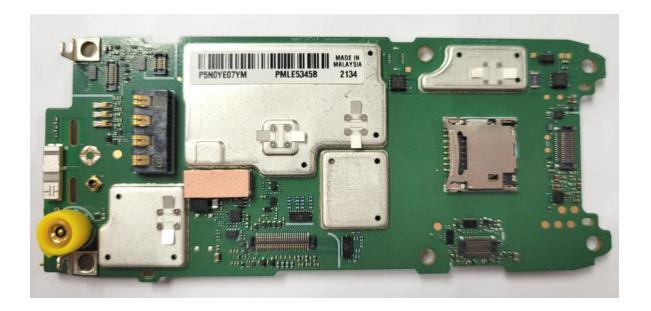
RF Board with Shields (Bottom), Model MXP600
