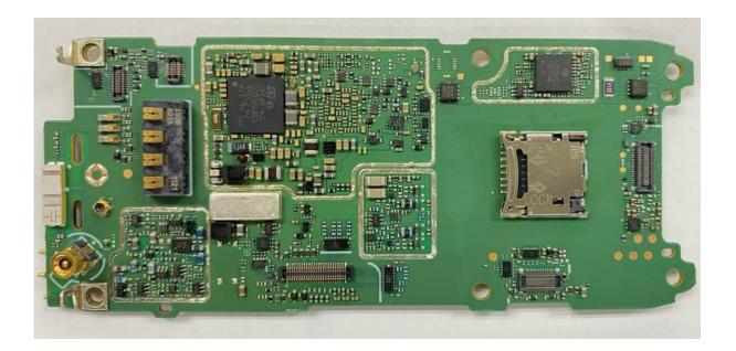
RF Board without Shields (Bottom), Model MXP600
