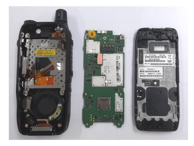
RF Board with Chassis and Housing (Back Side), Model MXP600
