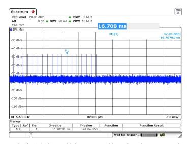
Peak of -47.04dBm, with losses at combiners factoring antenna gain to be 15.81dB, therefore level going into antenna port is -62.85dBm which exceeds threshold level of -64dBm for successful detection.
