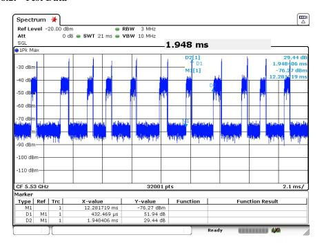
The resulting plot data was extracted and post processed, giving a duty cycle of 22.2%.
