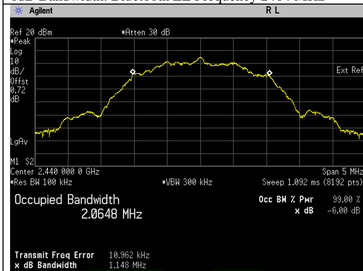
6dB Bandwidth. Bluetooth LE Frequency 2440 MHz
