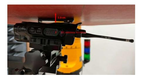
The BT maximum power of the device is 22.39 mW with 78% duty cycle, therefore the standalone Bluetooth transmitter operates at maximum time-averaged power:
