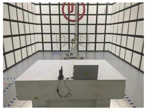
RADIATED SPURIOUS EMISSION SETUP ABOVE 1 GHz
