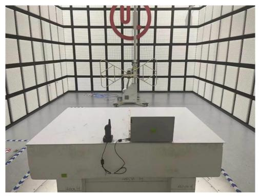
RADIATED SPURIOUS EMISSION SETUP ABOVE 1 GHz
