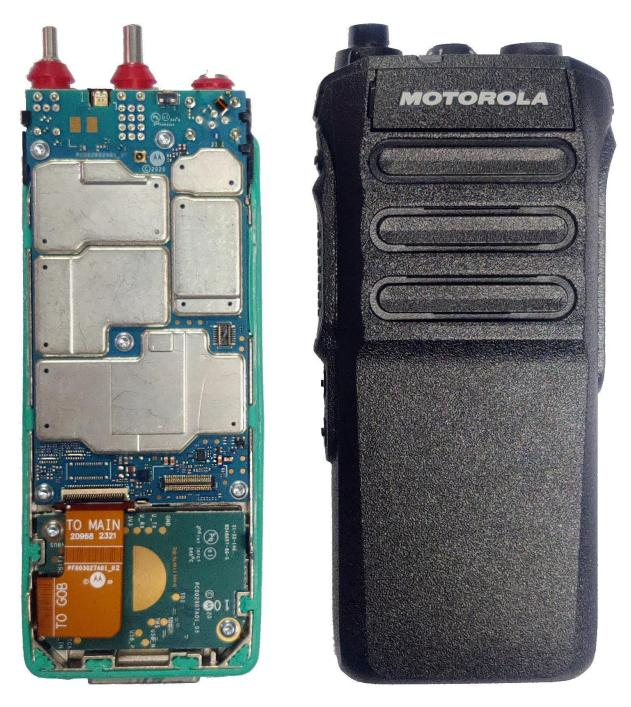
RF board <u>with</u> chassis and housing (front side) of NKP TIA Model
