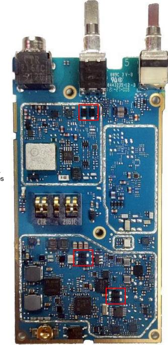
RF board without Shields (Bottom) of FKP TIA Model
