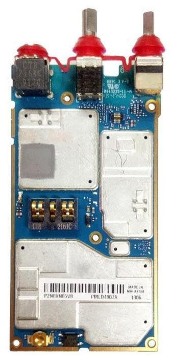
RF board with Shields (Bottom) of NKP TIA Model
