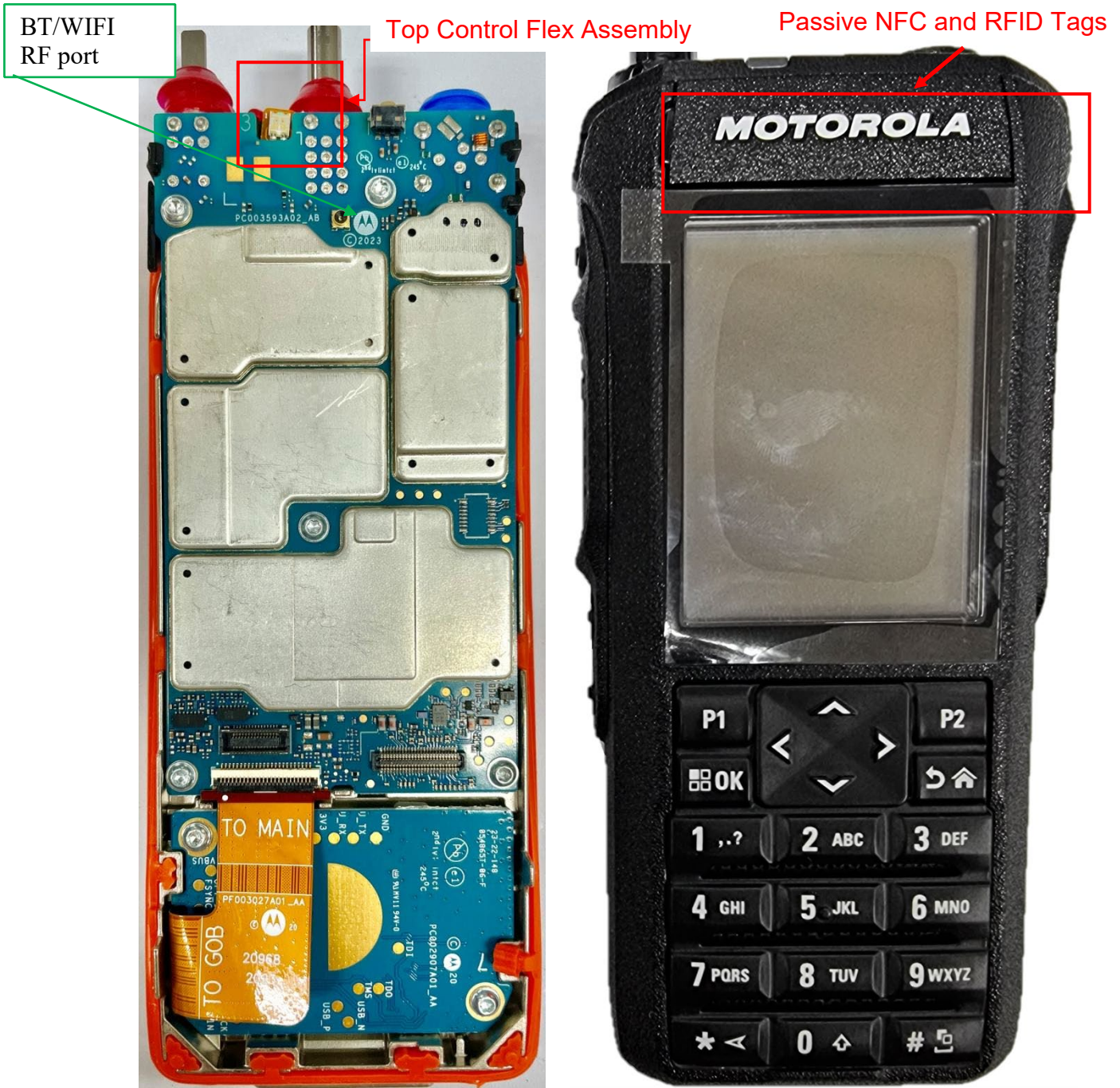
RF board with chassis and housing (front side) of FKP TIA/non-TIA Models
