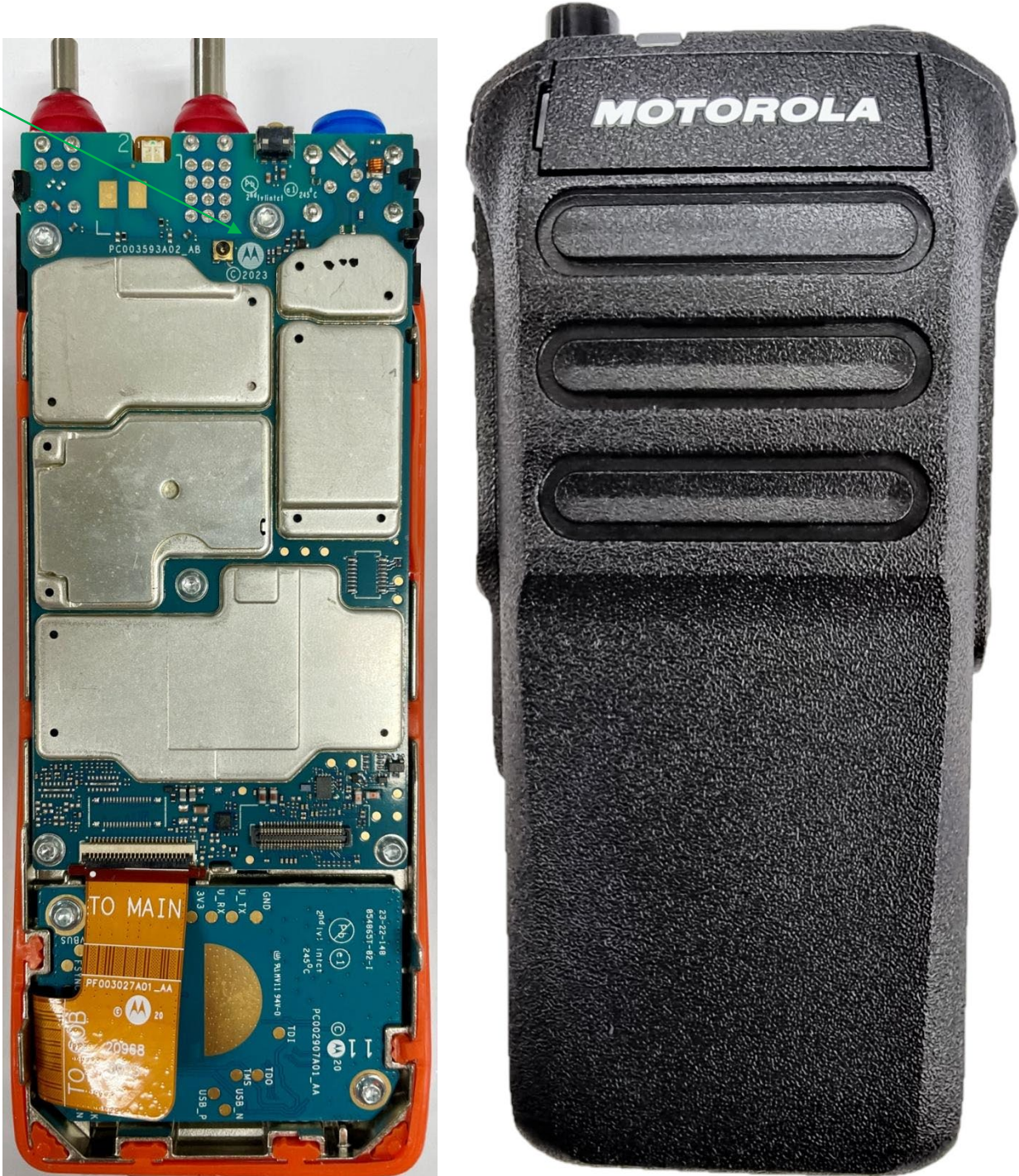
RF board with chassis and housing (front side) of NKP TIA Model
