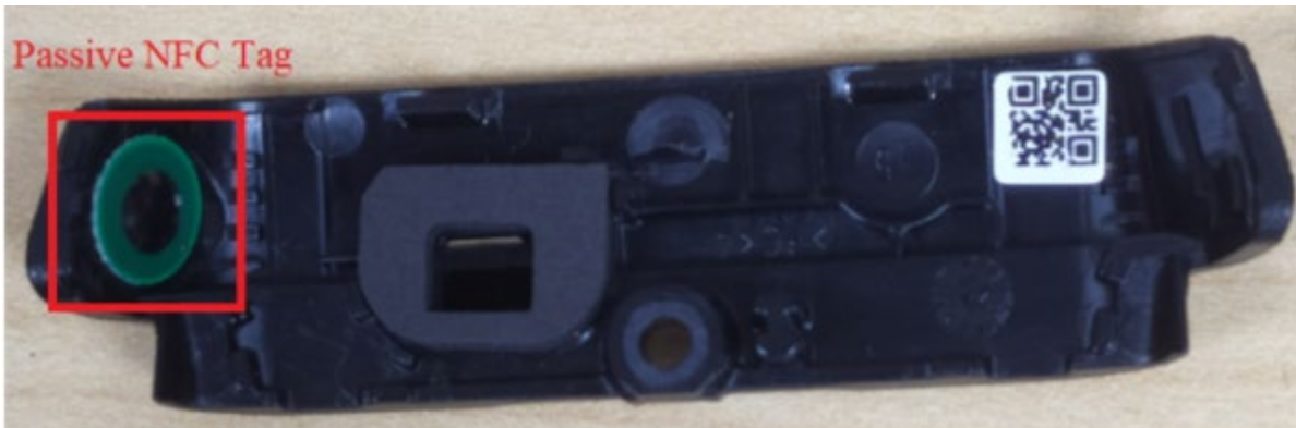
Location of the Passive NFC Tag at the Shroud of the FKP TIA/non-TIA Models
