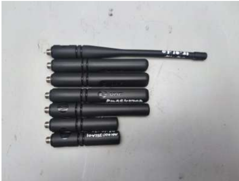
From bottom to top: AN000351A01, AN000350A01, AN000348A01, PMAE4070A, PMAE4071A, AN000389A01 and PMAE4079A
